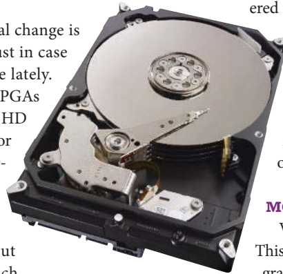
5. Seagate's Kinetic Terascale drive links 4 Tbytes of storage to two on-board Ethernet interfaces.
