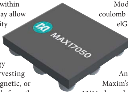
3. Maxim Integrated's MAX17050 high-accuracy battery fuel gauge uses the company's ModelGauge m3 algorithm to make continuous micro-corrections and eliminate sudden jumps in a battery's state of charge.
