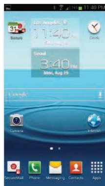
2. Green Hills Software and ViaSat are delivering military-grade security for Android smart phones and tablets. A little red lock indicates the locked apps in the secured version of Android. Tapping them runs them in the unsecured version of Android.
