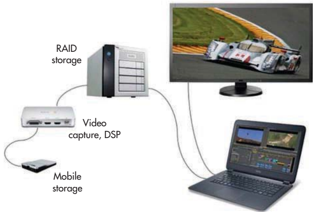
6. Designed to deliver 4K video, Intel's Thunderbolt 2 hardware interface combines the two previously independent 10-Gbit/s channels into one 20-Gbit/s bi-directional channel that supports data and/or display.
